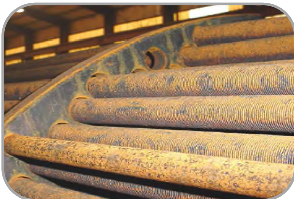
Typical Fretting in a Conventional S&T HEX
